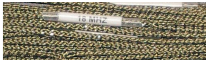
Closeup of the "Flexiweave" cord and also the frequency labels
